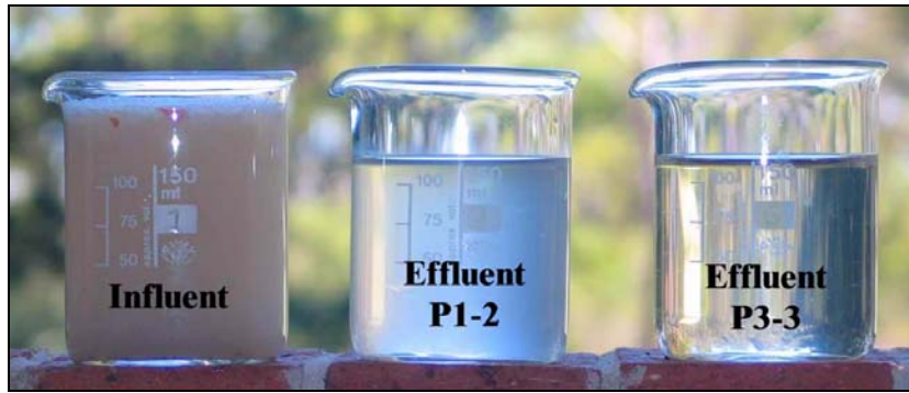
Figure 4.4: Water quality across biofilter units: influent, primary effluent (P1-2) and final effluent (P3-3)
