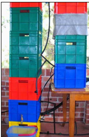
Figure 2.1: Greywater System Pilot Plant Unit Setup
